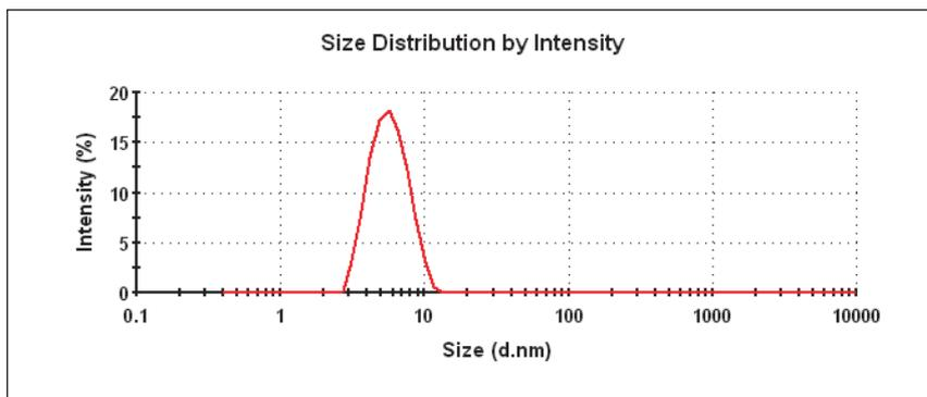
**Figure 2:** Intensity particle size distribution obtained for uncoated ferro oxide nanoparticles dispersed in hexane
