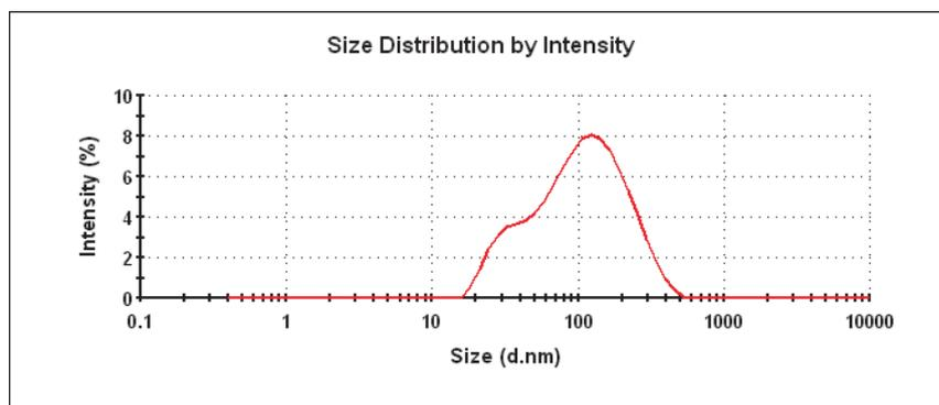
**Figure 3:** Intensity particle size distribution obtained for coated ferro oxide nanoparticles dispersed in hexane
