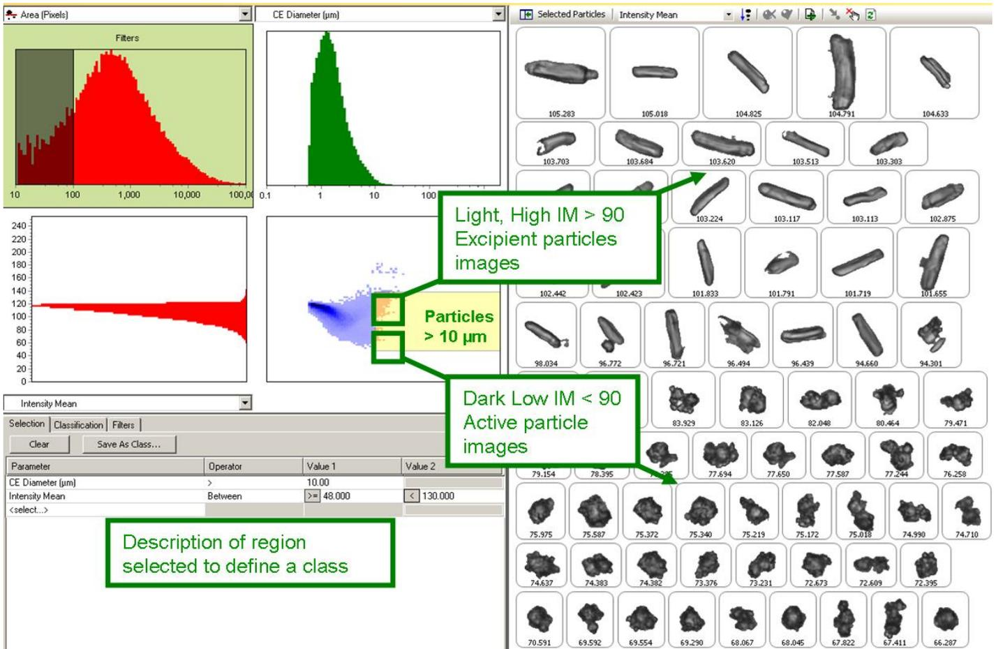
Figure 2: Screen shot of the Morphologi G3's scattergram feature and selected particle images sorted in terms of Intensity mean
