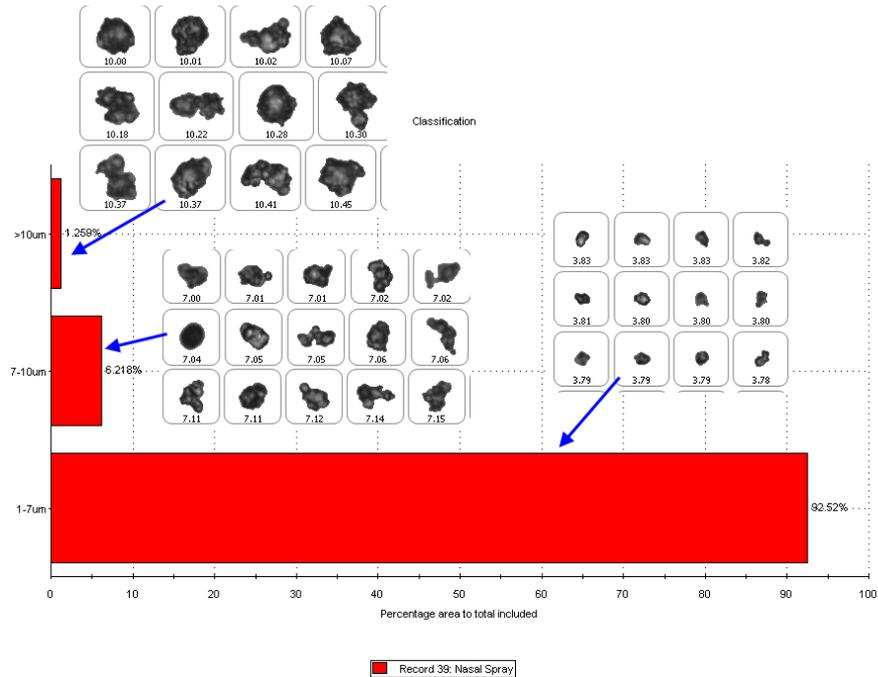
**Figure 1:** Classification chart showing the proportion of active particles found in each size class along with example particle images
