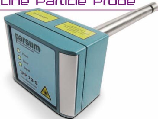
Spatial filter velocimetry from 50 to 6000 $\mu$ m
