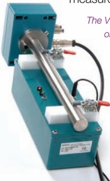
*The VK consists of a rotating disc inside a casing on which the probe is attached. Set into the rotating disc are 3 calibration pins with certified diameters of 150, 1000 and 2000µm.*
