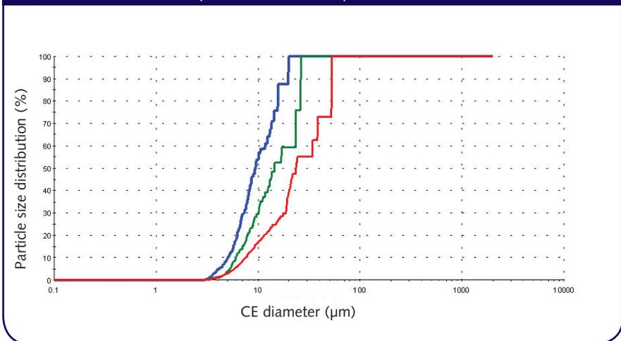
*The example data included here show how morphologically directed Raman spectroscopy can successfully differentiate between clinker in a sample and other components, such as limestone and slag, to generate component-specific size distribution data for each one.*
