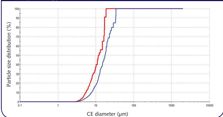
Figure 4: size distribution analysis for a CEM II/B-M (S-L) 42,5 N sample shows that within the sample the limestone (blue) has the finest particle size distribution, followed by the slag (green line), with the clinker (red line) present as the coarsest particles
