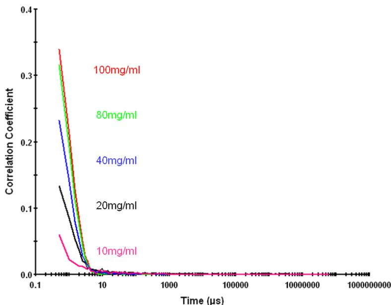
**Figure 5:** Correlation functions obtained from measurements of various concentrations of vitamin B1; 100, 80, 40, 20 and 10mg/ml respectively.
